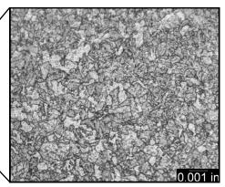
When examining large components that cannot be easily moved, in-place metallography is used for microstructural and crack evaluation. In-place metallography, combined with replication, allows us to examine a component's microstructure without removing a sample from the component. The same techniques can be used on small specimens when standard preparation methods are difficult or impossible.
